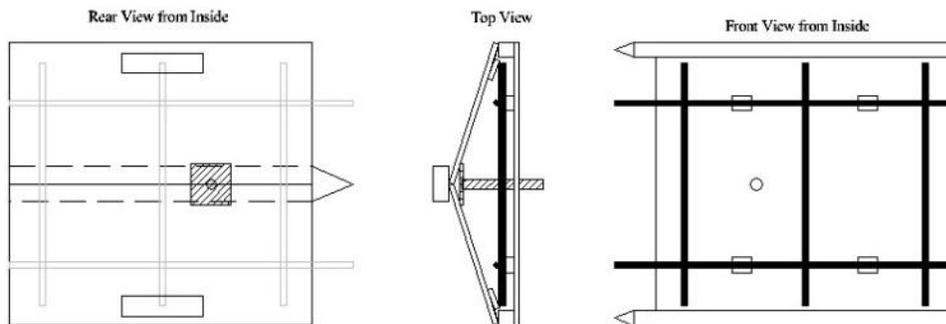
**Figure 12 - Inside View of Ground Anchor Form**
