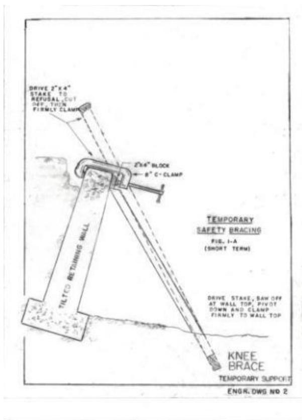
Figure 1 - Safety Bracing (Short Term)
